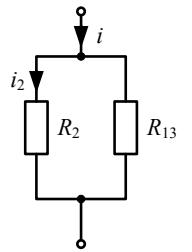
$$R_{13} = \frac{R_1 \cdot R_3}{R_1 + R_3} = \frac{6 \cdot 24}{6 + 24} = \frac{144}{30} = 4.8 \Omega$$
