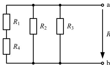
$$R_5 = R_1 + R_4 = 10 + 20 = 30 \Omega$$
