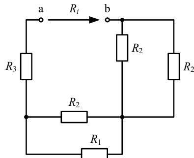
$$R_i = R_3 + \frac{R_1 \cdot R_2}{R_1 + R_2} + \frac{R_2 \cdot R_2}{R_2 + R_2} = 20 + \frac{5 \cdot 10}{5+10} + \frac{R_2}{2} = \\ = 20 + \frac{50}{15} + 5 = \frac{425}{15} = \frac{85}{3} \Omega$$
