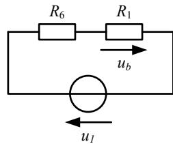
$$R_6 = R_3 + R_4 + R_5 = 20 + \frac{10}{3} + 5 = \frac{85}{3} \Omega$$
