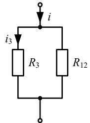
$$R_{12} = \frac{R_1 \cdot R_2}{R_1 + R_2} = \frac{6 \cdot 24}{6 + 24} = \frac{144}{30} = 4.8 \Omega$$
