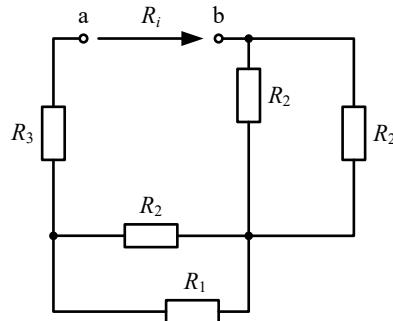
$$\begin{aligned} R_i &= R_3 + \frac{R_1 \cdot R_2}{R_1 + R_2} + \frac{R_2 \cdot R_2}{R_2 + R_2} = 20 + \frac{5 \cdot 10}{5+10} + \frac{R_2}{2} = \\ &= 20 + \frac{50}{15} + 5 = \frac{425}{15} = \frac{85}{3} \Omega \end{aligned}$$
