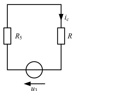
$$R_5 = \frac{R_2 \cdot R_4}{R_2 + R_4} = \frac{10 \cdot 10}{10 + 10} = \frac{100}{20} = 5 \Omega$$
