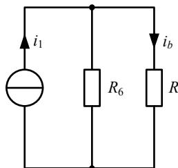
$$\frac{1}{R_6} = \frac{1}{R_2} + \frac{1}{R_3} + \frac{1}{R_5} = \frac{1}{30} + \frac{1}{30} + \frac{1}{30} = \frac{3}{30} = \frac{1}{10} \text{ S}$$
