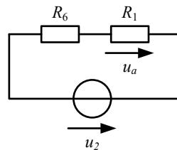
$$R_6 = R_3 + R_4 + R_5 = 20 + 5 + \frac{10}{3} = \frac{85}{3} \Omega$$
