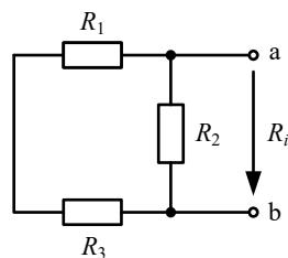
$$R_4 = R_1 + R_3 = 2 + 8 = 10 \Omega$$
